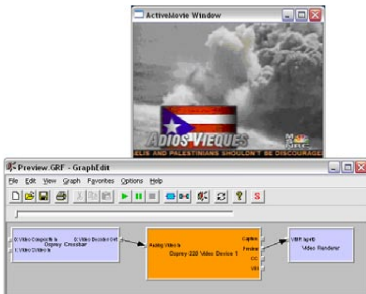
1 A common filtergraph based on the Osprey AVStream driver, with a preview window.
